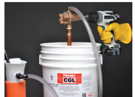
CGL pumped into duct using an LP-D5 pump
