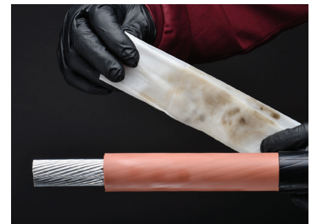
Residue from cleaning
