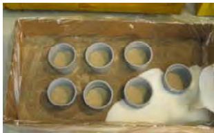
InstaGrout™ is mixed and poured
