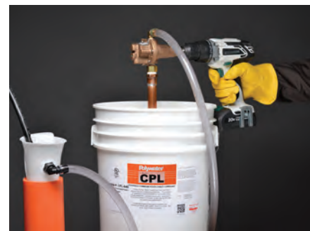
CPL applied using the LP-D5 pump
