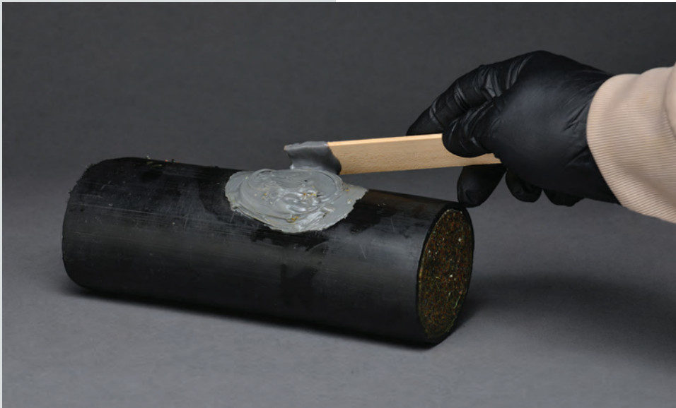
AirRepair applied to a telco cable
