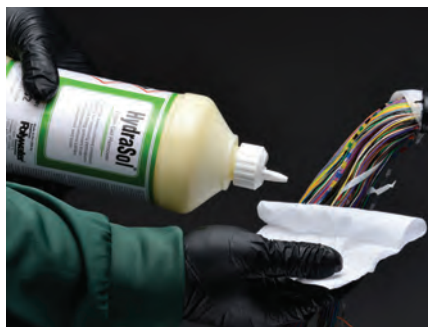
HS-32 applied to towelette for cleaning
